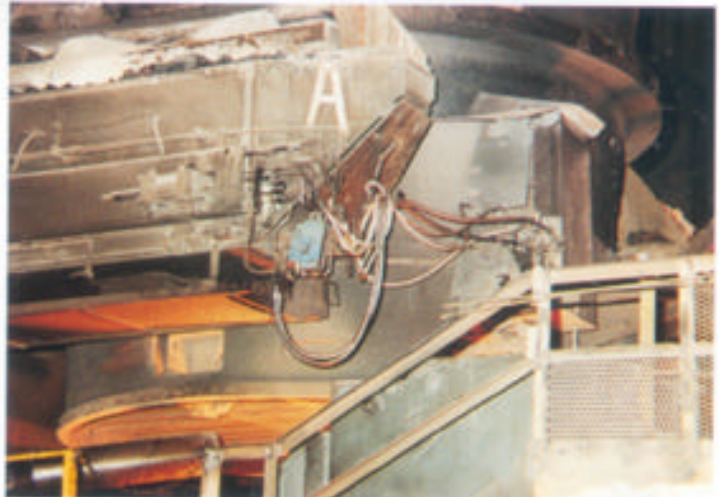
GSM Hydraulic Hose from the turret arm, activating the slide gate on the ladle.
