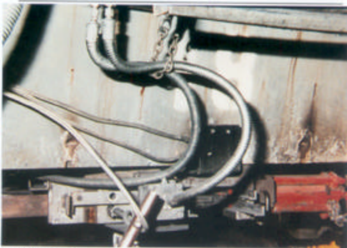
GSM Hydraulic Hose activates slide gate system on the tundish.
