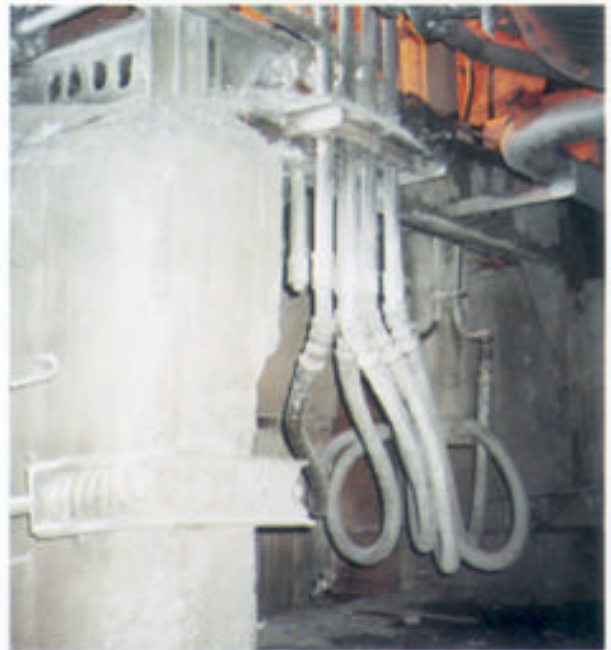
GSM Tilt Cylinder Hydraulic Hose resists sparks and slag from furnace above.
